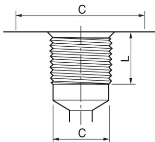
*ISO Internal Parallel Pipe Thread*
