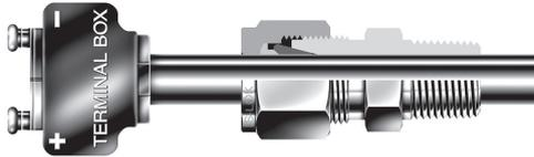
S-LOK thermocouple connector has no shoulder nor sizing angle inside the fitting; the features enable thermocouple to go through the fitting's thread end.
