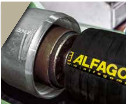
4. Coupling insertion on the hose
