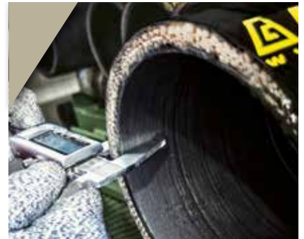
3. Hose thickness measurement is taken to obtain the correct calibrated crimping diameter
